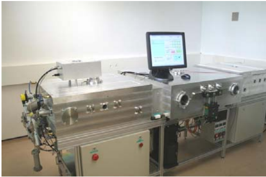
Figure 1: Automated thin-film silicon dual-chamber deposition system on the basis of oerlikon solar's KAI-M plasma box (photo: IMT).
