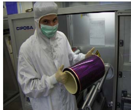
Figure 2: Multi-pass single-chamber processing at VHF-Technologies (photo: IMT).
