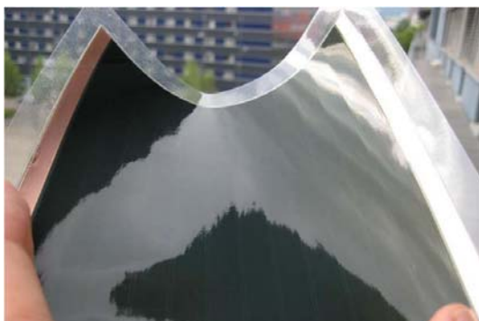
Figure 3: A prototype of monolithically inter-connected CIGS module on polymer film (photo: ETHZ).
