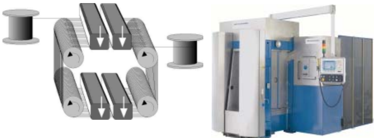
Fig. 2.3 Left: The principle of multi-wire sawing - the workpiece is pushed into the wire web, which is wound from one side to the other and transports the cutting medium into the saw-gaps. Right: The DS 262, capable of slicing 2 m of accumulated length in one single run, producing over 4'500 wafers / run.
