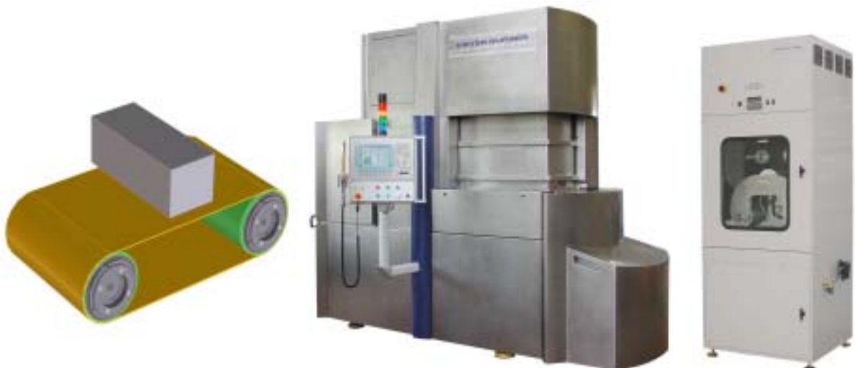
Fig. 4.2 Concept of the two-roller technology (left). The easy accessibility of the DS 265 is clearly visible (centre). This enables a rapid conversion from SiC to diamond slurry or diamond wire. The DWT multi-wire saw is ideally suited for pure diamond wire pv slicing experiments.
