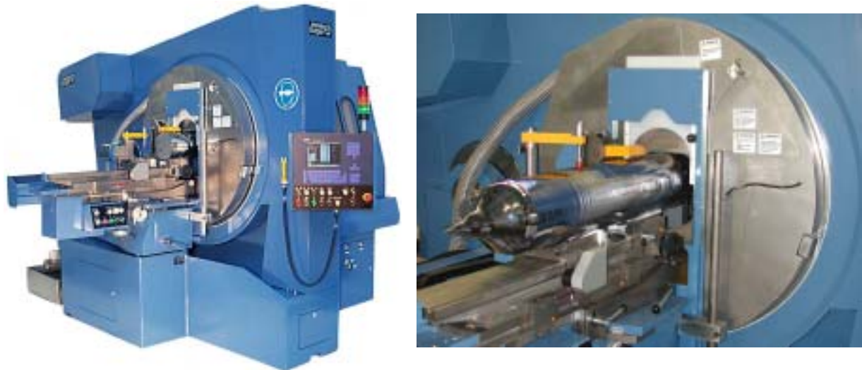
Fig. 2.1 An 8" single crystal ingot being cropped on an ID-hole saw (ID: Inner Diameter) TS207.
