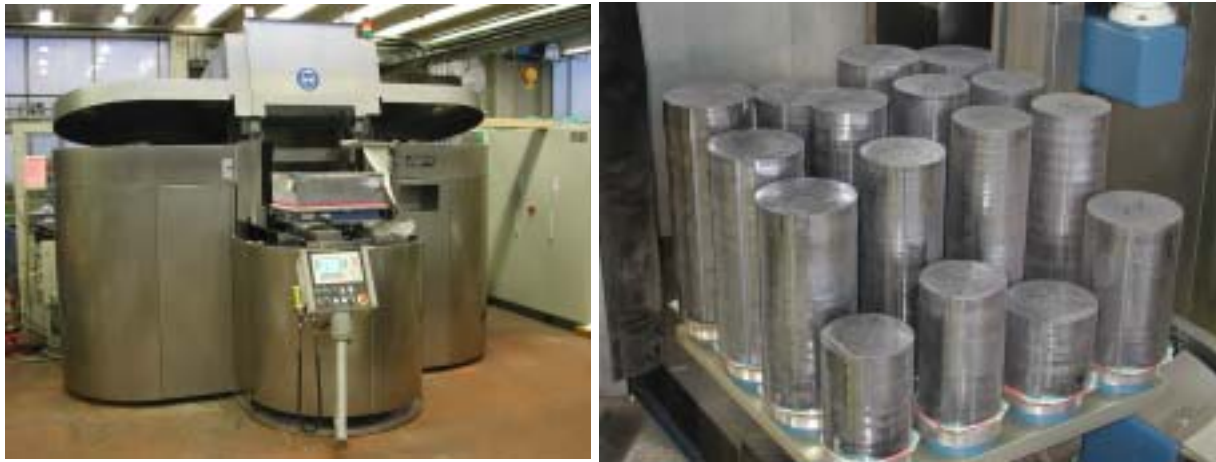
Fig. 2.2 Photo of the BS800 with a poly silicon ingot to be cut into bricks (left). Photo of the BS 805, loaded with single crystals for squaring (right).
